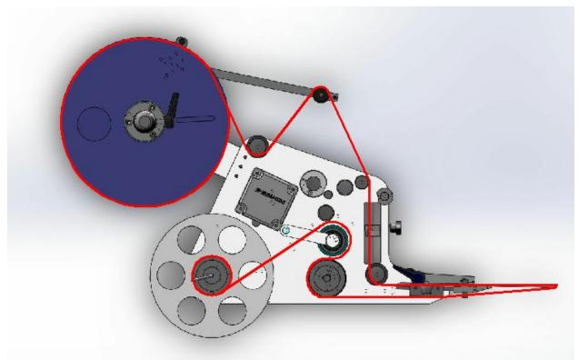
The diagram indicates the correct path for threading the labels.
