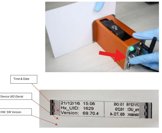
Figure 11. Print Test Result
