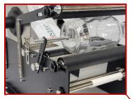
Use the bottle guide to ensure consistent placement of labels.
