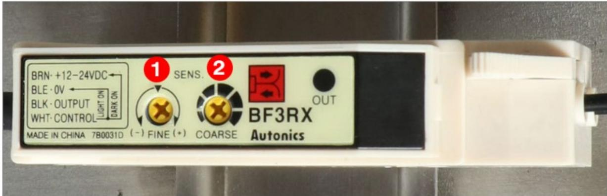
1. To adjust the sensitivity of the bottle sensor, place the bottle underneath the sensor and adjust the screws clockwise or counterclockwise until the indicator light turns on.
